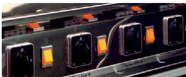
quadro comandi con accensioni indipendenti control panel with independent ignitions
